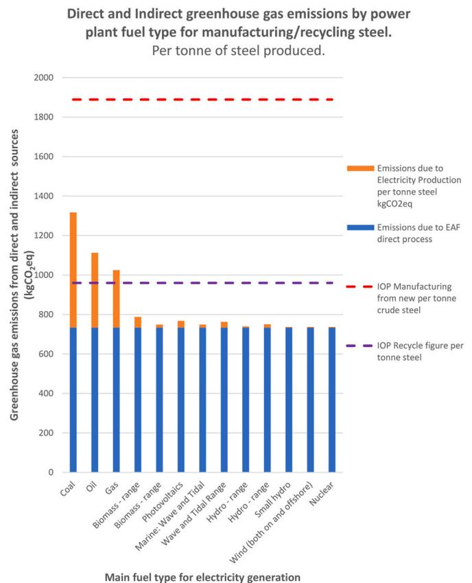
Fig. 7. Carbon footprint of EAF process plus the carbon footprint of electricity generated to produce 1 tonne of steel. (Parliament (2020), Chesnokov et al., 2014), Navas-Anguita et al. (2019).
