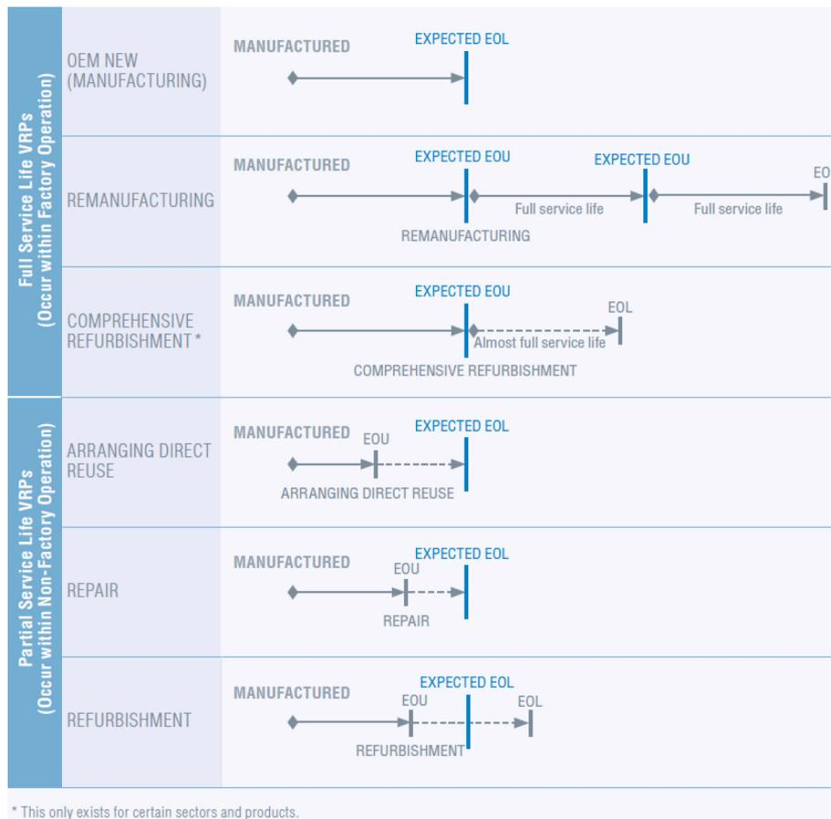
Fig. 11. Description of value-retention potential of Value-Retention Processes (VRPs). The original equipment manufacturer (OEM) refers to the items manufactured, assembled and installed during the construction of a new product.
