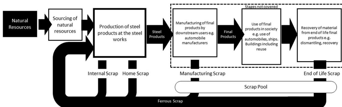
Fig. 10. Schematic diagram of the life cycle of steel showing included stages as well as those excluded. From ISO 20915:2018 (2018).
