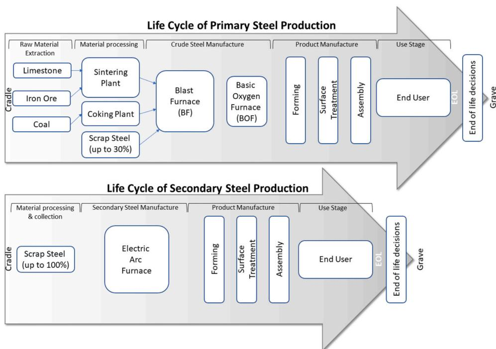
Fig. 4. A simplified life cycle of primary and secondary steel production and product manufacturing showing the cradle-to-grave approach taken here. Adapted from Stahl (Accessed Dec 2020).
