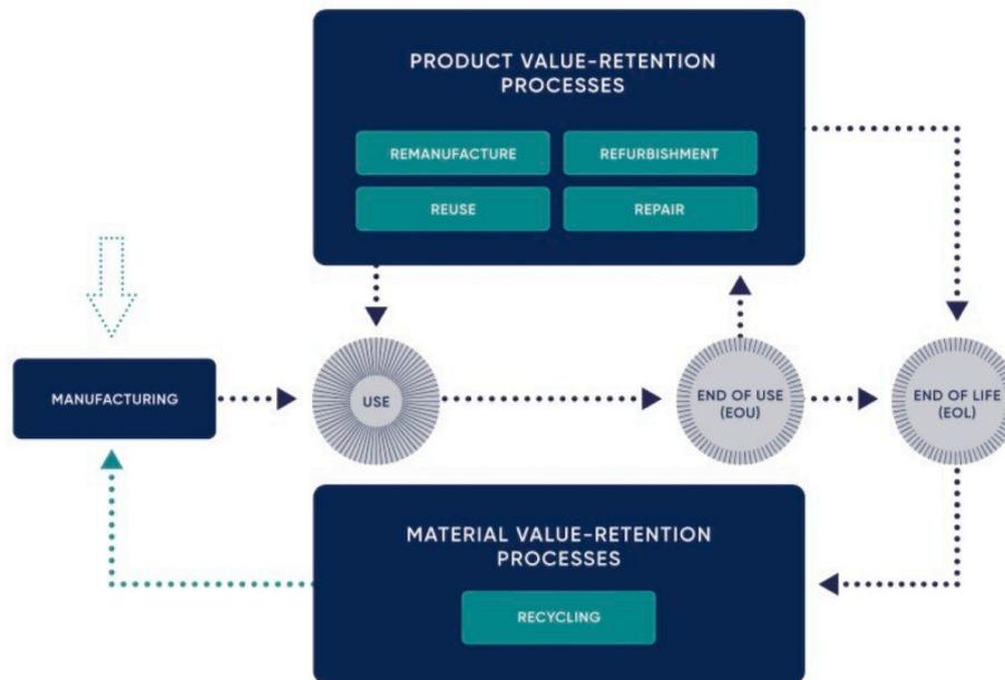
Fig. 12. Product life cycle using the principles of value-retention to select the most effective strategy for retaining the highest value from the materials and products. From Oakdene Hollins (2020).
