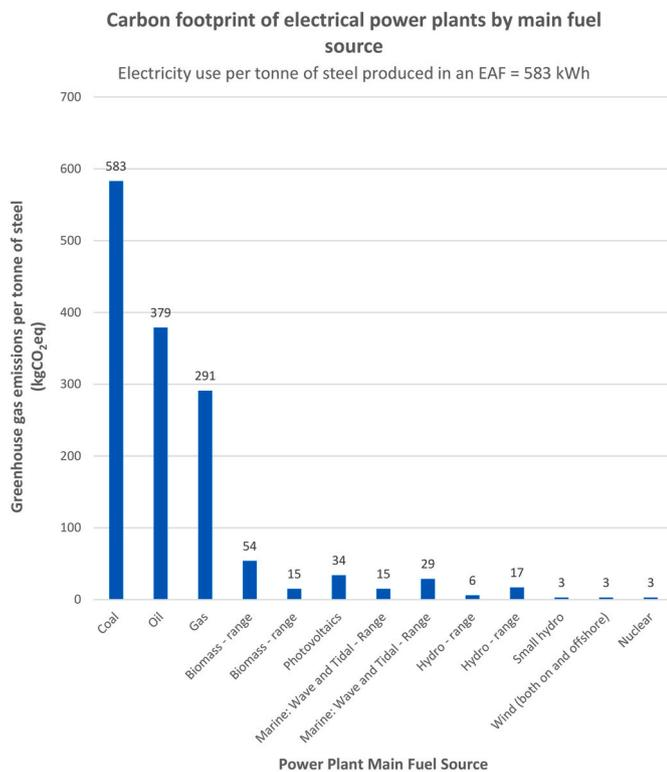
Fig. 6. Carbon footprint of power plants by fuel source for producing electricity for use in an Electric Arc Furnace EAF (<https://www.parliament.uk/globalassets/ets/documents/post/postpn268.pdf>, 2020), EAF figure of 583 kWh from Navas-Anguita et al. (2019).
